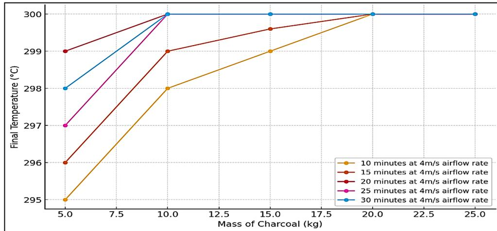
Fig. 8. Mass of charcoal plotted against temperature for 10, - 30 minute operation at 4m/s airflow rate.
