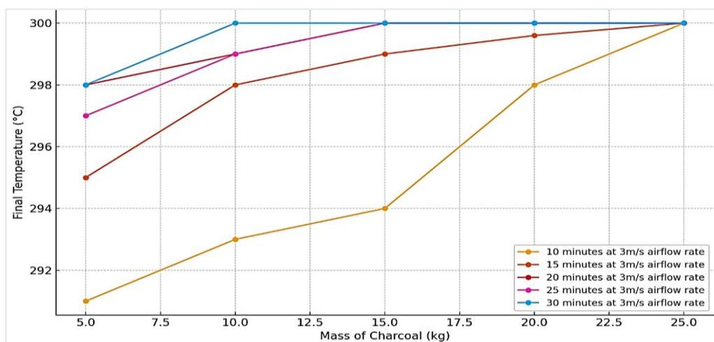
Fig. 7. Mass of charcoal plotted against temperature for 10-30 minute operation at 3m/s airflow rate.
