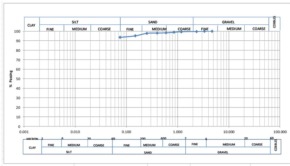
Fig. 4. Grain size distribution curve.
