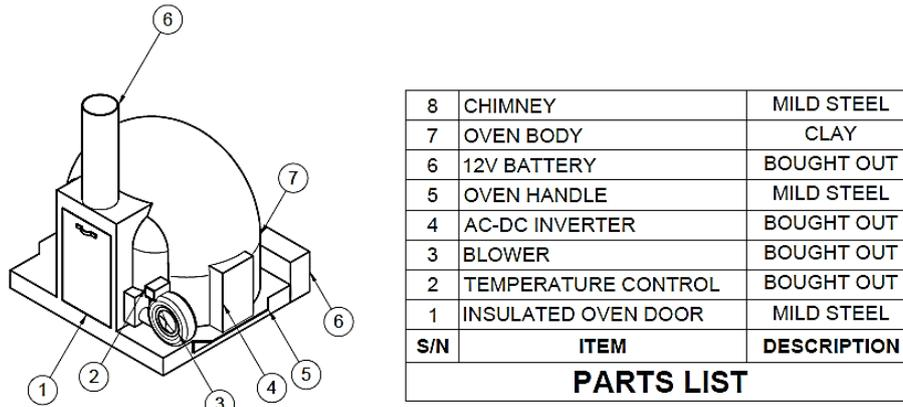
Fig. 1. CAD model of the automated clay oven.
