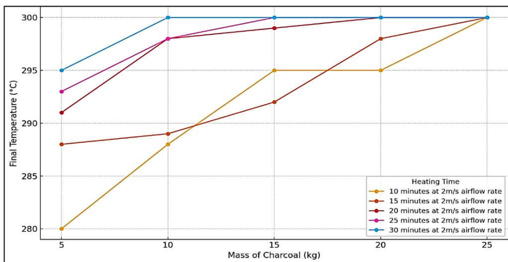
Fig. 6. Plot of temperature and mass of charcoal for 10-30 minute operation at 2m/s airflow rate.
