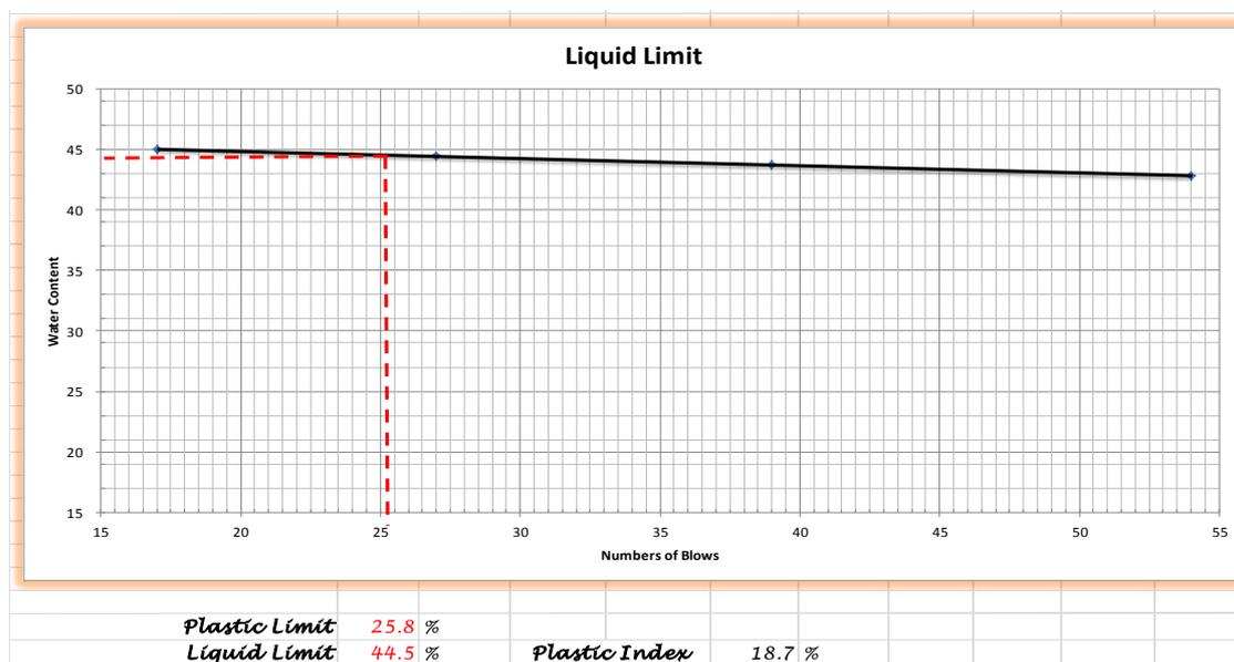
Fig. 5. Result of liquid limit test.
